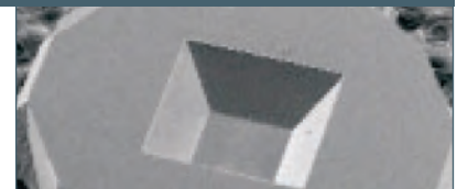
SEM image of a DuraSiN™ Film (taken from the back side)
