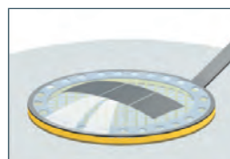
5. The grid holds to the LOOP by surface tension.
