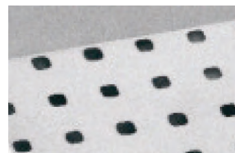
SEM image of a DuraSiN™ Mesh (taken from the back side)
