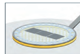
6. Lower the LOOP to the filter paper to remove water.
