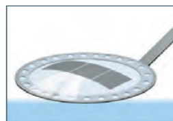
3. Gently lift up the LOOP with the sections in a droplet of water
