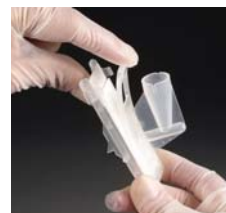
Clip top of funnel and base together.
